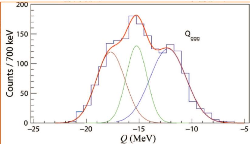
Fig. 2. (color online)  $Q$ -value spectrum for the  $^{14}\text{C} \rightarrow {}^{10}\text{Be} + \alpha$  breakup reaction on a proton target, obtained from the present measurement. The  $Q_{\text{ggg}}$  peak is related to the final particles all in their g.s.. The other two peaks correspond to the exit  ${}^{10}\text{Be}$  in its first excited state (3.36 MeV) and its four adjoining excited states around 6 MeV.
