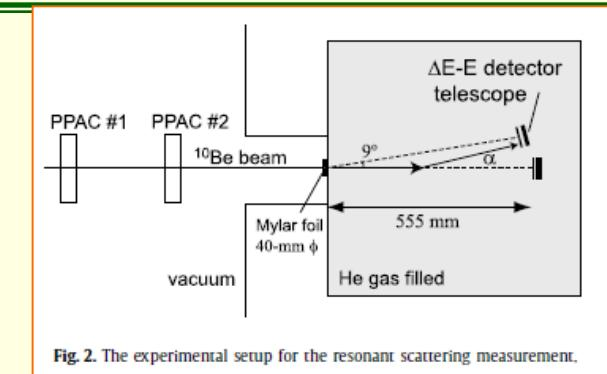
Fig. 2. The experimental setup for the resonant scattering measurement.
