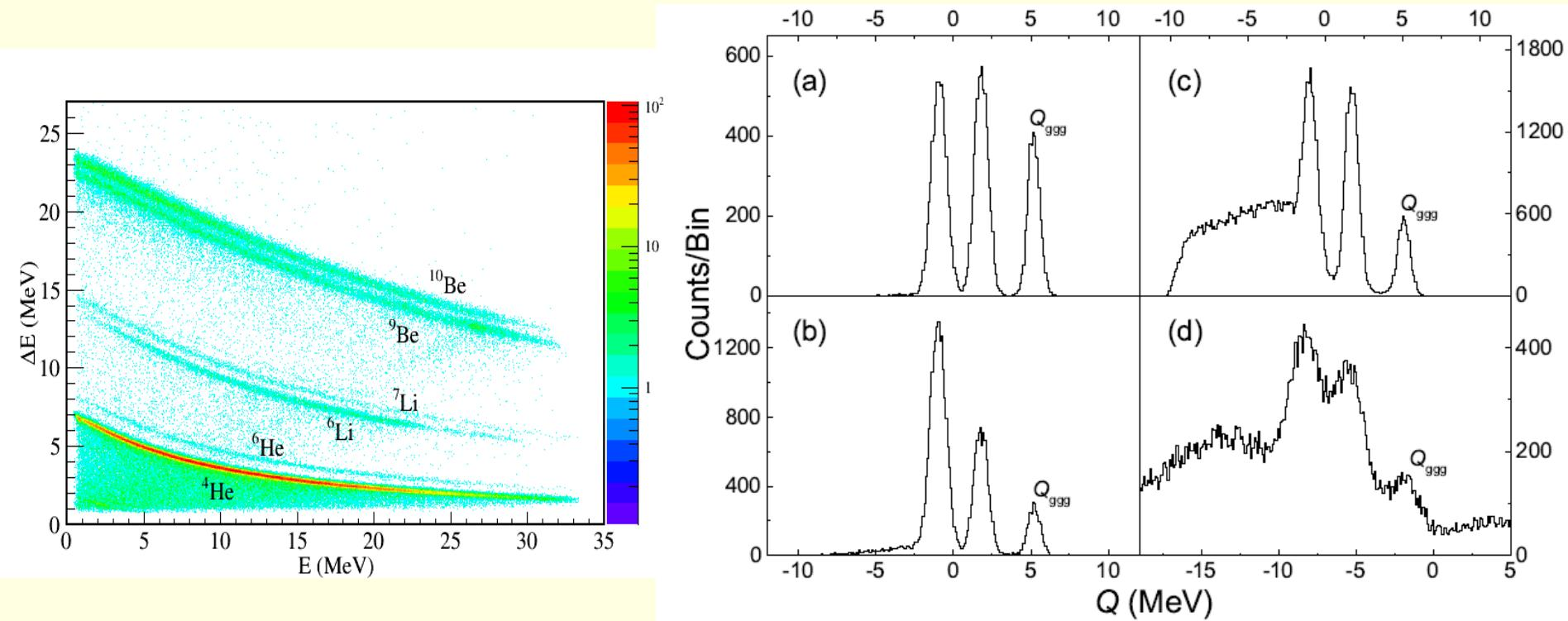
FIG. 1:  $Q$ -value spectrum from present experiment for different data sets with: (a) identified  $^{10}\text{Be}$  and identified  $\alpha$  in U0/D0 telescopes; (b) identified  $^{10}\text{Be}$  and unidentified  $\alpha$ ; (c) identified  $\alpha$  and unidentified  $^{10}\text{Be}$ . Spectrum (d) comes from previous  $^7\text{Li}(^9\text{Be}, \alpha ^{10}\text{Be})^2\text{H}$  experiment [11].
